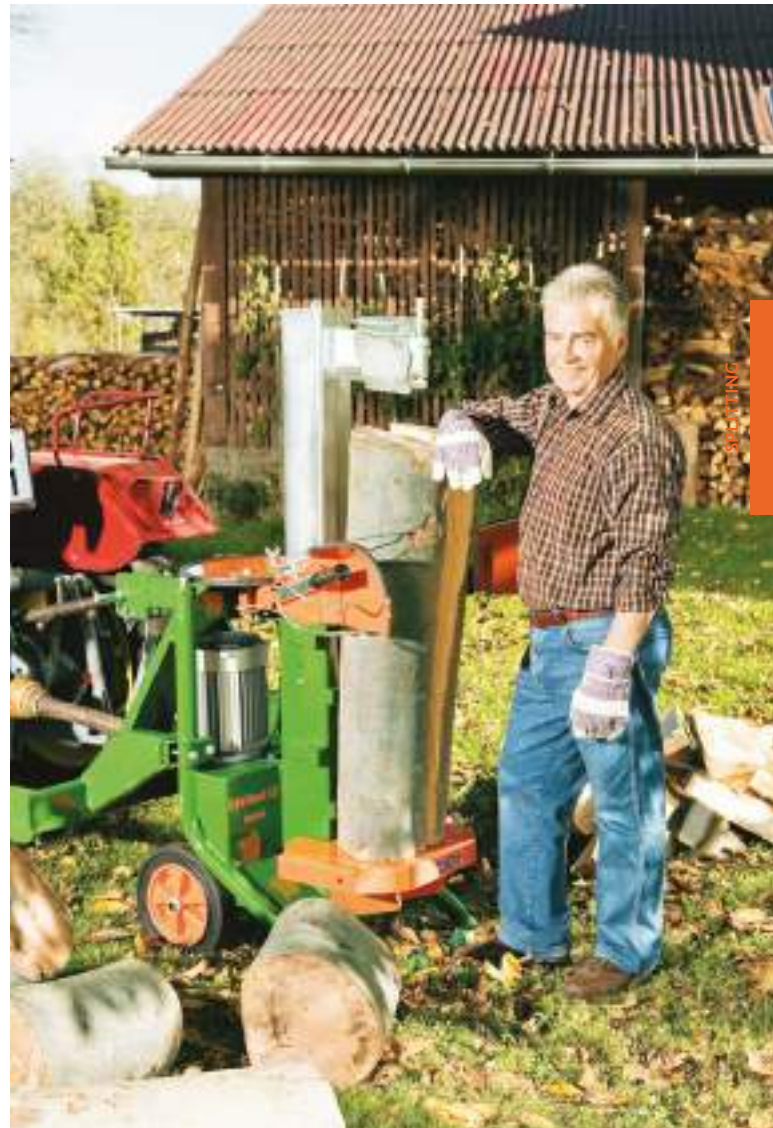
With the height-adjustable splitting table, you can also produce metre-long logs with SpaltAxt Special.
