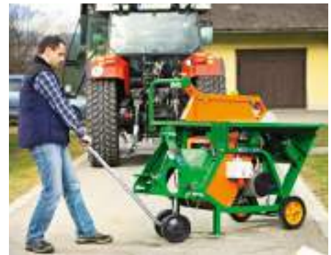
Transport aid for easy manoeuvring on farms for the tilting table saw with PTO drive.
