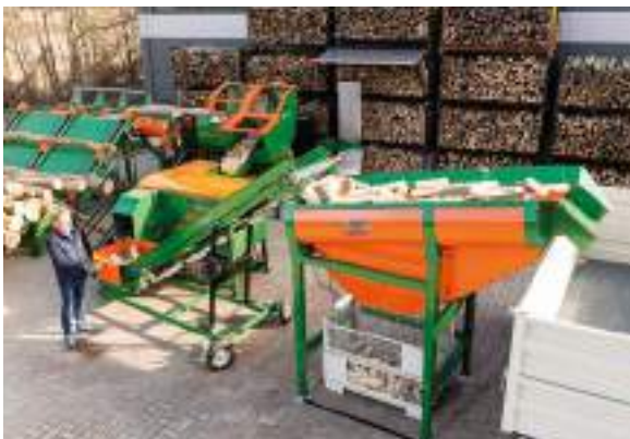
LogFix L waste wood is transported to a suitable container or an optional conveyor belt.
