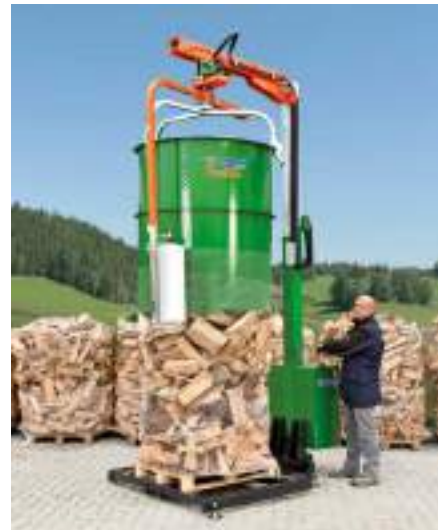
The drum itself does not rotate and is pulled upwards hydraulically.
